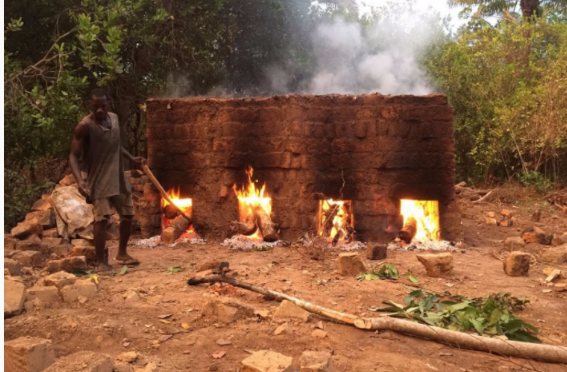
It was a close call but God held the rains off enough so we could start the bricks burning. We're praying that the fire is just right and we don't lose too many bricks.
